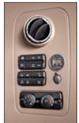
A wall-mounted console controls all of the sleeper conveniences, including HVAC and the dome light.
