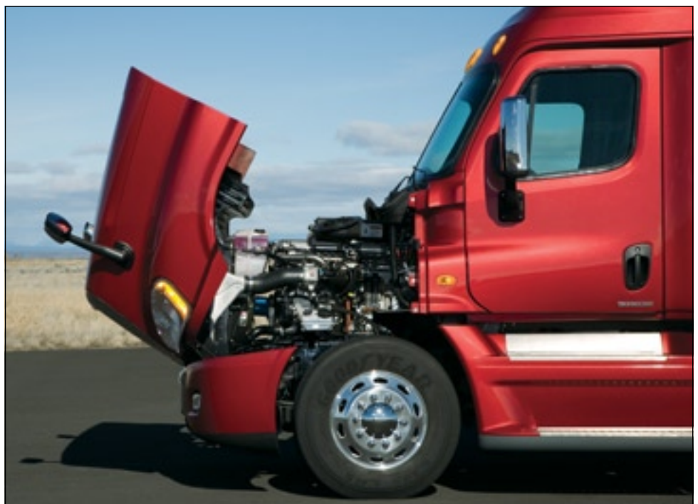
The hood opens wide; the engine and see-through fluid reservoirs are placed in easy view and reach for daily inspections and routine maintenance.
