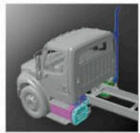
**CLEAR BACK-OF-CAB TAILPIPE**Clear left-hand and right-hand transmission
