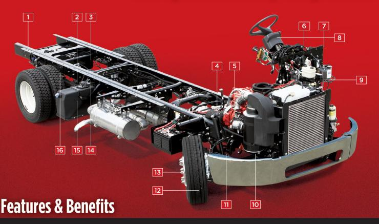
The MT-55 heavy-duty chassis offers a gross vehicle weight rating of between 20,500 and 30,000 lb. and can accept bodies with more than 1,500 cubic feet of volume. With a massive payload capacity of up to 19,000 lb., the MT-55 is the perfect choice for high-payload applications like newspaper delivery, utilities and tool trucks.
